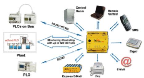
To handle the changes of I/Os and PLC variables the 'Process' subsystem is part of the Tixi Device firmware. The following picture shows how it triggeres the event processing.
