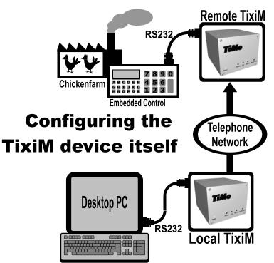
In this configuration the desktop PC controls the remote Tixi Alarm Modem by means of the TiXML protocol. To do this the following steps are required:
