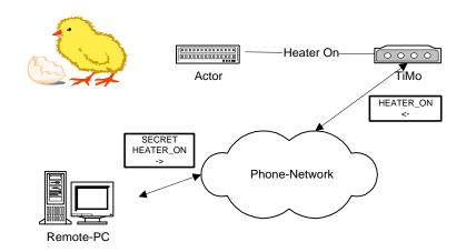
The Tixi Alarm Modem has an extension module with output ports (for example with a module address of C42). At the output ports, some actuators are connected by an electrical signal line (for example a heater).
