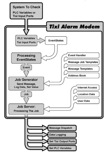
At first there is a "**system to check**" which may be a **PLC** connected via serial port or some switches and measure instruments connected to the Tixi Alarm Modem **I/O-Ports**. The configuration of PLCs is documentated in a separate "PLC TiXML Manual". The processing of I/Os or PLC variables is explained in **chapter 6**. A not supported PLC may control the Tixi Alarm Modem via TiXML-commands, e.g. the DoOn-Command to activate alarms (see. **chapter 2.4.9.1**)
